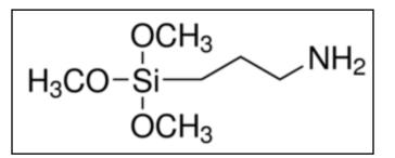
Figure 2. The structure of 3-aminopropyltrimethoxysilane.
